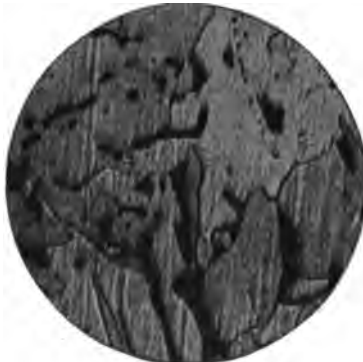
Fig. 30. Burnt Steel showing Cracks between Crystals
